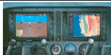
Garmin G1000 Instrument Panel of a Cessna 172 Skyhawk
