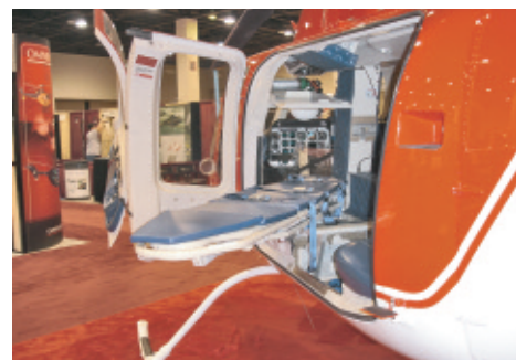
Bell 407 Helicopter with Spectrum air ambulance equipment.
