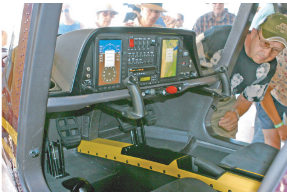
Cessna's SkyCatcher will be equipped with the new Garmin G-300, which is still under development.
