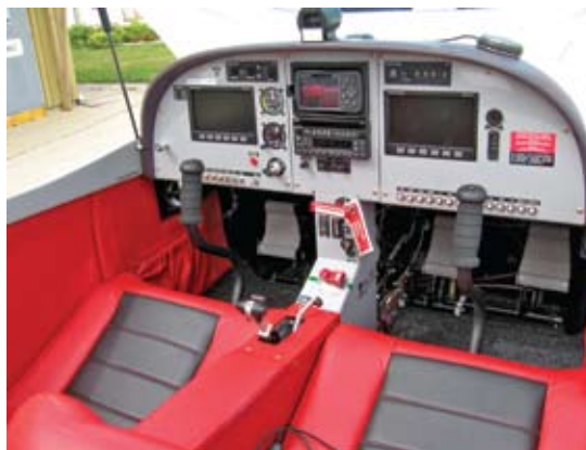
The top-of-the-line glass panel-equipped cockpit of the Piper Sport LTD, complete with autopilot and ballistic recovery parachute.
