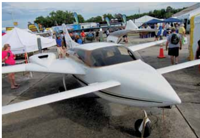
Looking a bit like the little brother of a Beech Starship, Velocity Aircraft debuted a new twin-engine version of the speedy four-place canard.
