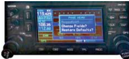
After entering the updated flight plan into the Garmin 430, the "Menu Button" on Nav-Page 1 will bring up the cross-fill option that can be selected with the "Enter Button."
