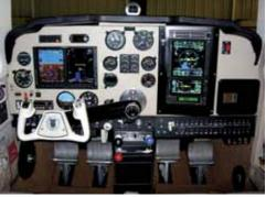
Avionics interfacing problems can be isolated and resolved through persistence. In this example, there was a design error in the Garmin GMA 350 audio panel when interfaced with the King KFC 150 auto pilot. When the aircraft was on auto pilot and on an ILS approach, the Beechcraft A36 Bonanza would oscillate as soon as it captured the glideslope signal. The problem was fixed with a wiring change.
