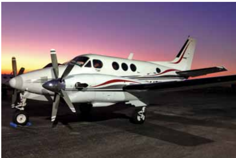
Beechcraft King Air C90 with GE H80 turboprop engines.
