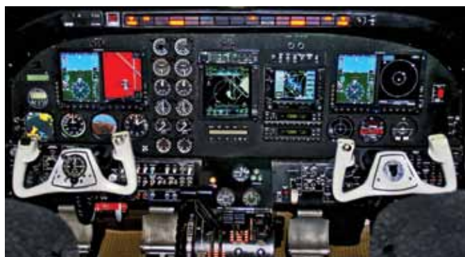
State-of-the-art Garmin glass panel with dual G600 PFD/MFD displays.
