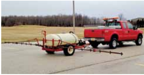
Some GA airports are applying liquid deicing chemical with a converted agricultural sprayer.
