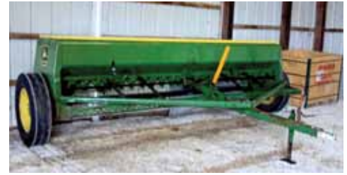
A farm grain drill can be used to spread dry deicing chemicals.
