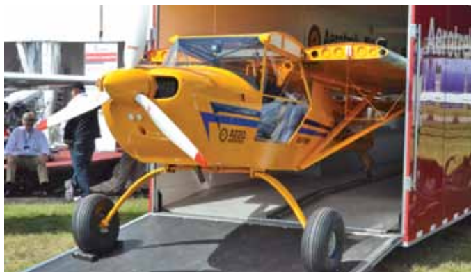
The wings of the Aerotek fold for easy storage and transport.
