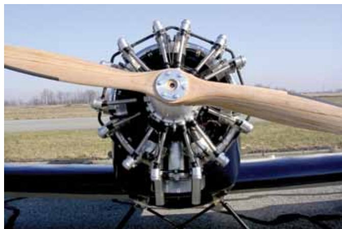
The Aerolab LoCamp prototype is powered by the Rotec R2800 radial engine.
