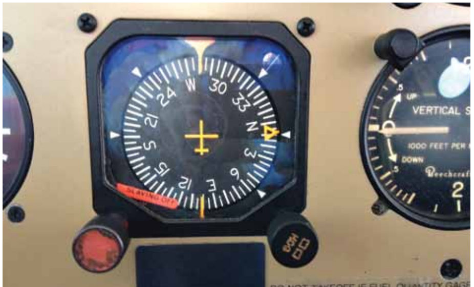
A slaved heading indicator eliminates having to constantly make directional adjustments.
