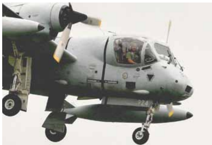
The big and speedy “Grumman Mohawk” is capable of impressive short-field operations, with a slow approach speed and reversing propellers.
