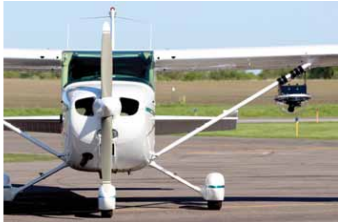
Cinematographer, James Aarestad, mounts his camera on a three-axis gyroscopically stabilized gimbal, which keeps the camera steady to within .001 degrees.
