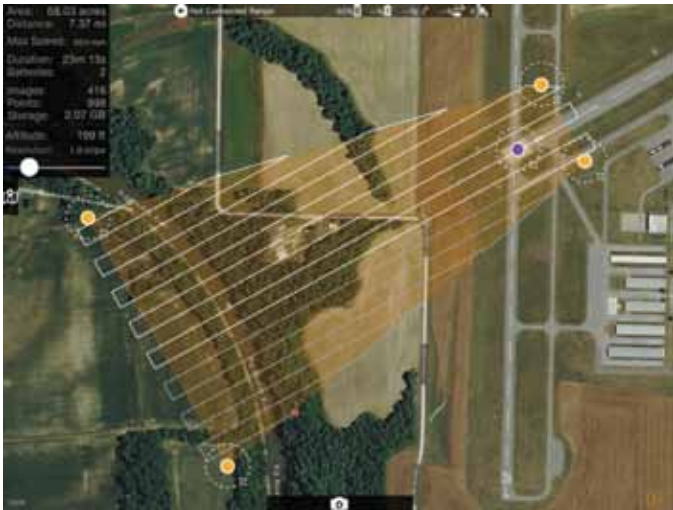
Flight path flown to evaluate obstructions in the approach to Runway 6 at Southern Illinois Airport (KMDH), Carbondale, Ill.
