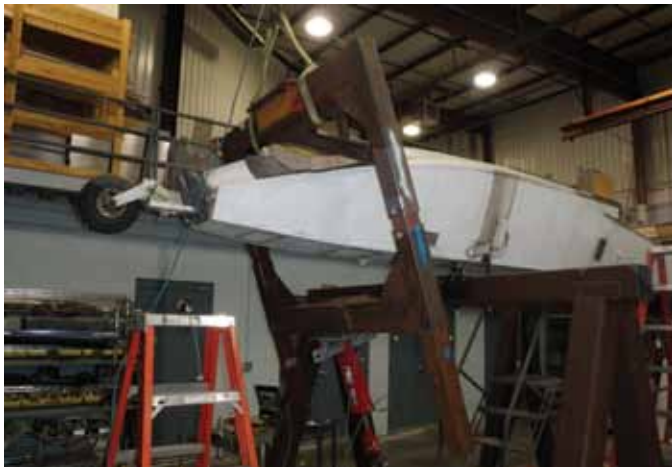
Bow load application to a float during static structural testing. Wipaire Photo
