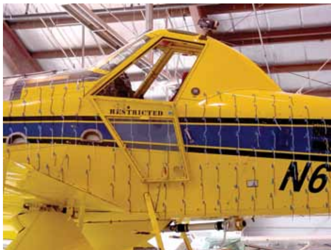
Tufted fuselage of an AT-802A to aid in flow visualization. Wipaire Photo
