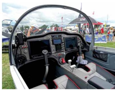
Bob and Joan Zaleski's Sling 2 features dual Garmin G3X Touch™ Flight Displays, a Garmin GTN 635 Touchscreen Navigator, a Garmin G5 Electronic Flight Instrument System (EFIS), and a Garmin autopilot.
