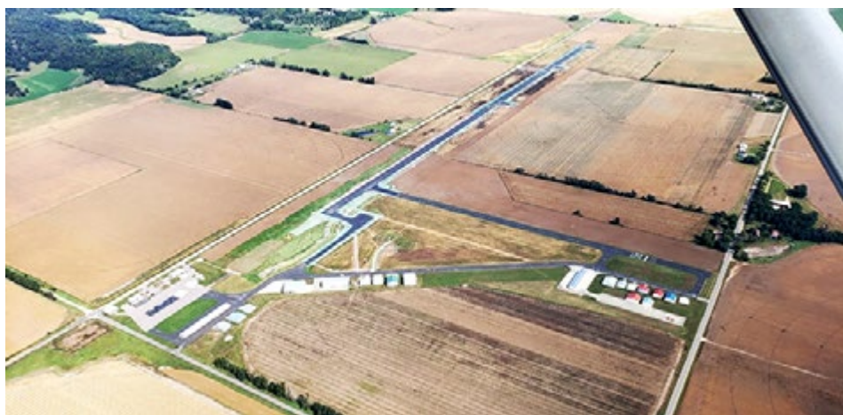
Newly raised and reconstructed Runway 9/27 at Tri-County Regional Airport, along with water management improvements. Photo courtesy of Westwood
