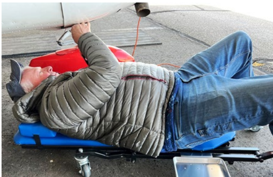
The AeroCreeper lowers to 5 1/4 inches and extends up to just over 20 inches.
