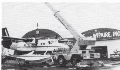
A MARKAIR airline Twin Otter is mated with floats for the first time. The Wipline 13000 floats were engineered especially for this aircraft. Photo courtesy of Wipaire, Inc.
